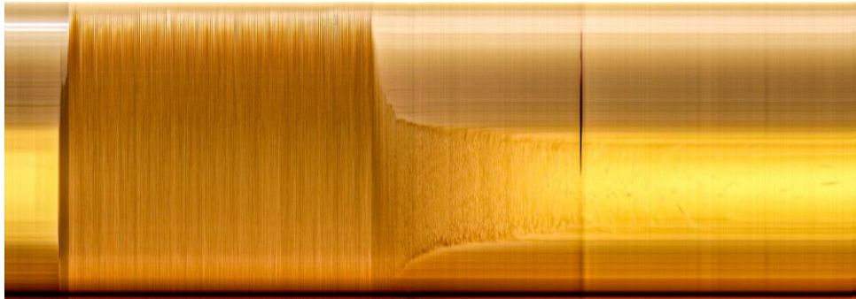
Figure 1 Visualisation of the timeline of suspension formation through stirring and its sedimentation after switching off the impeller.
