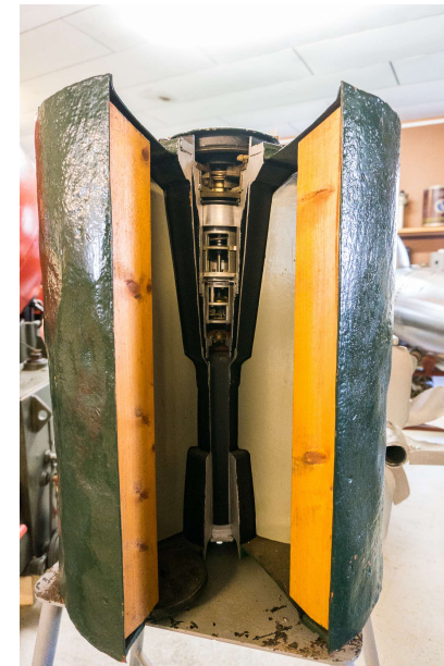
German depth charge Type I ('Wasserbombe') [1]
